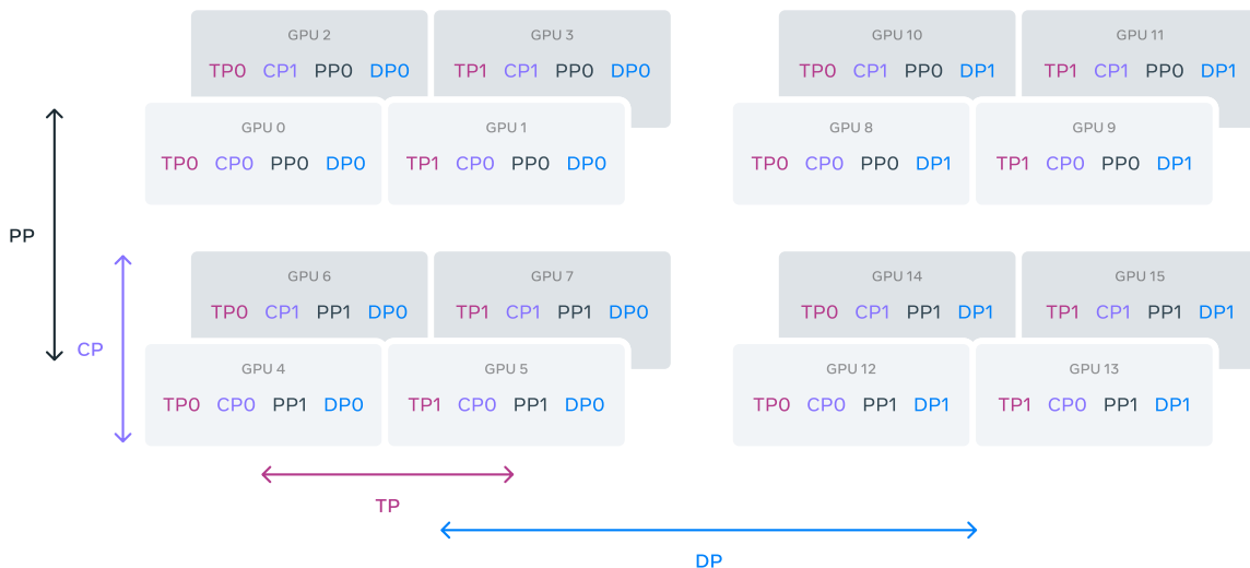
Figure 5 Illustration of 4D parallelism. GPUs are divided into parallelism groups in the order of [TP, CP, PP, DP], where DP stands for FSDP. In this example, 16 GPUs are configured with a group size of |\text{TP}|=2 , |\text{CP}|=2 , |\text{PP}|=2 , and |\text{DP}|=2 . A GPU’s position in 4D parallelism is represented as a vector, [D_1, D_2, D_3, D_4] , where D_i is the index on the i -th parallelism dimension. In this example, GPU0[TP0, CP0, PP0, DP0] and GPU1[TP1, CP0, PP0, DP0] are in the same TP group, GPU0 and GPU2 are in the same CP group, GPU0 and GPU4 are in the same PP group, and GPU0 and GPU8 are in the same DP group.
